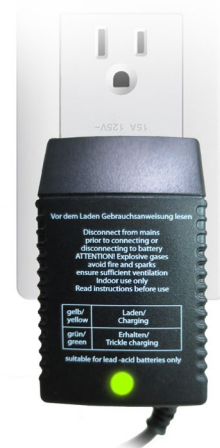
Green indicates charging complete
