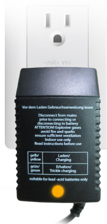
Yellow indicates charging
